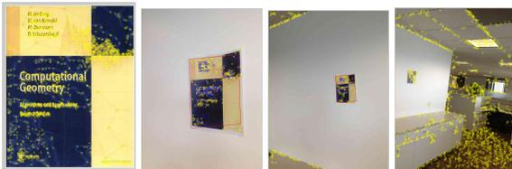
**Fig. 2:** Covers2 dataset Images. From left to right, Model Image (2516 features) , Test image ( Close-60 deg, 9/416 features matched), Test Image (Moderate -45 deg, 32/262 features matched) , Test Image ( Far- 60 deg, 0/1848 features matched).
