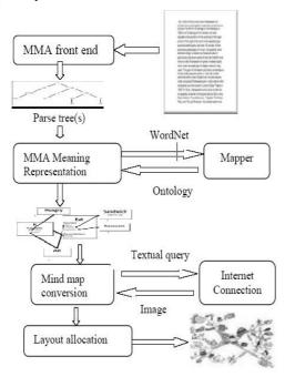
Fig. 5: The implementation Phases of the MMA system with the Inputs and Outputs.
